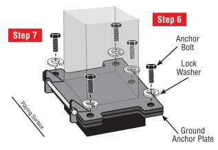
**Step 9:** Snug tighten the five anchor bolts, then check goal assembly with a level and inspect visually to determine if it is parallel and plumb to the playing surface.
