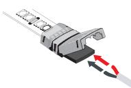
2. Strip 3/4" grey sheathing back, DO NOT strip red and black wires, insert the two wires into the corresponding wire channel on long side of connector. Matching Red wire to (+ or WW) side of tape, Black wire (- or CW) side of tape.
