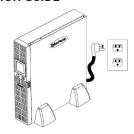
is equipped with an auto-charge feature. When the UPS is plugged into an AC outlet, the battery will automatically charge whether the UPS is turned on or off.
