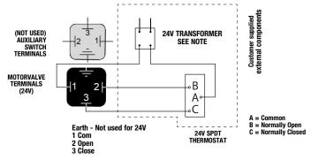
NOTE: ¼" - 2" EMVII-6400SS-24-40 will operate with a 40 VA transformer. Thermostat must be capable of handling amp rating at stall.
