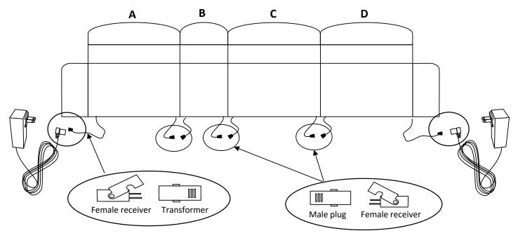
STEP 5: Connect wall plug transformers into a nearby outlet, still making sure it is clear of the metal base.
