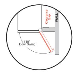
THE DOOR STOP IS SET AT  $110^{\circ}$  BUT CAN BE RESET TO  $90^{\circ}$  OR  $140^{\circ}$ .
