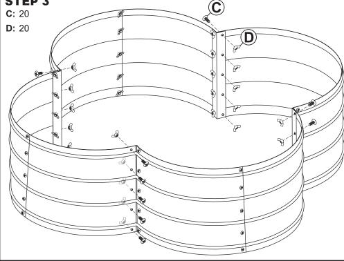
Align the four sets of panels and loosely fasten each section using the remaining Bolts (C) and Wing Nuts (D), as shown.
