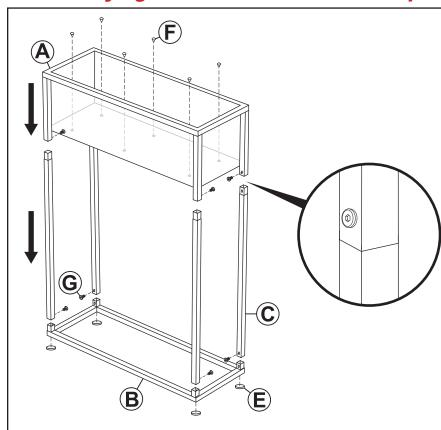
Apply four Protective Feet (E) to the bottom of Base (B).
