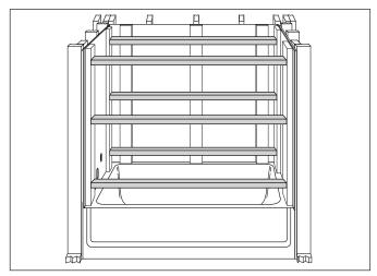
4. Insert (wedge) blocks or cross braces between the front to rear panel braces and the back panel braces. These blocks or braces must apply pressure to the back panel to hold it in place.
