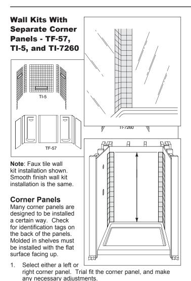
**Note**: Corner shower wall kits only have one corner panel. Install it with the flat surface of the molded in shelf facing up.
