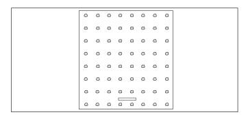
Install the back panel, overlapping the corner side panels.
