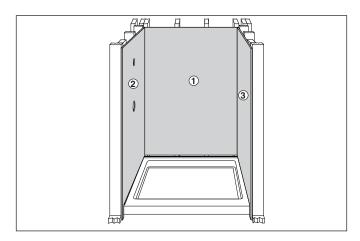
To prevent possible water (wicking affect) damage to the wall, install the wall board with a 1/2 inch gap above the bathtub or shower floor side lip, the front edge of the bathtub or shower floor, and the room floor.
