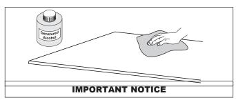
Do not use oil-based cleaners, such as mineral spirits, to clean the panels. The oil in the cleaner will prevent the panel from properly adhering to the wall.
