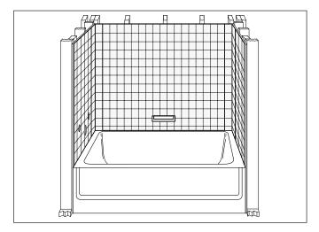
**Note**: Any gaps between the bottom of the panels and tub ledge will be filled in with caulking in a later step.
