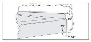
Apply a coat of water or oil-based primer/sealer to all the surfaces of the cement board or greenboard (follow the manufacturer's instructions). Allow the primer to dry
