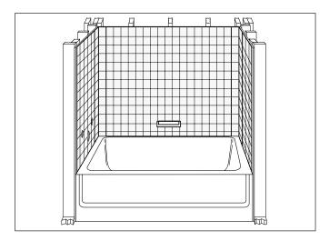
**Note**: Any gaps between the bottom of the panels and the tub ledge will be filled in with caulking in a later step.
