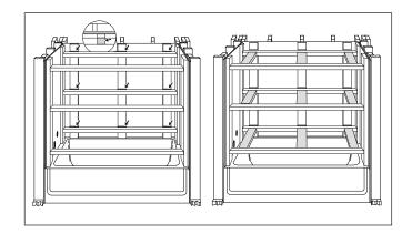
For corner shower wall installation use the illustrated bracing design.
