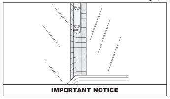
Model TI-7236, TI-7248, and TI-7260 Shower Wall Kits. The sides of the corner panels are different widths. One side is 5 inches wide and the other is 7 inches wide. The orientation of the corner panel will affect the allowable width of the wall dimensions. Refer to the illustration and chart for proper orientation.
