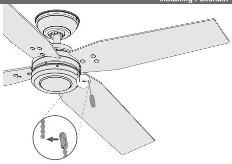
Installing the pull chain pendant - Attach the pull chain pendant to the short chain coming from the switch housing.
