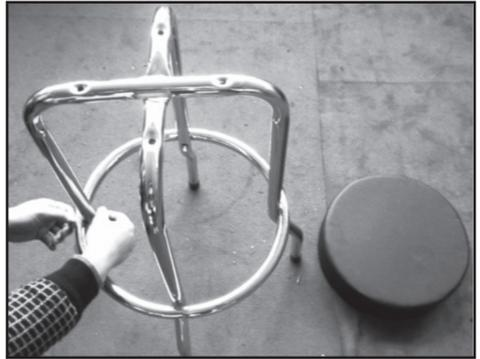
2. Slide the larger ring over the legs and align the holes. Slide the sleeved hex head screw into the hole and a hex head screw through the other side and tighten down using the supplied hex wrench. Repeat for the other holes.
