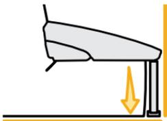
**⚠ Do not use the load leg on top of vehicle storage compartments. Review your vehicle owner's manual. Do not use the load leg if it does not reach the floor of your vehicle. When not in use, the load leg must be stored under the base.**
