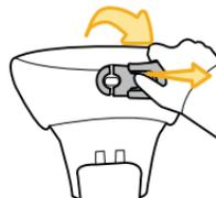
**With Your Thumb, Pull Down Locking Lever to Expand Attachment Openings**
