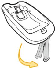
The load leg is stored under the base. This is an optional feature.
