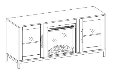
TOP PANEL FITS UP TO MOST 65in/165.1cm DIAGONAL FLAT PANEL TVS MAXIMUM LOAD 80lb/36.3kg.
