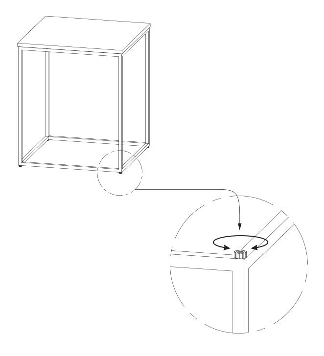
Note: Levelers on the bottom of the base can be adjusted if floor is uneven.
