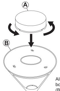
Align Base (A) with the bottom of Main Body (B), twist to secure.
