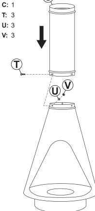
Align Flue (C) with the top of the main body and secure using three 1/4" x 3/4" Bolts (T), Washers (U), and Nuts (V).
