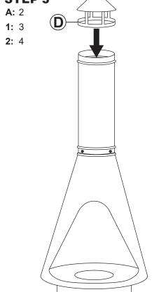
Place Rain Cap (D) on top of the flue.
