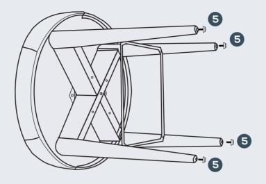
Check and tighten all the bolts again to ensure the stool is steady enough.
