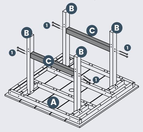
Attach Part C Side Rail between Part B Table Leg with 8 pcs of Hardware #2 Screw.
