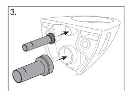
Remove pipes from wall and install into back of bowl. Make sure pipes are sealed thoroughly.
