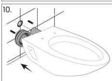
· Before mounting bowl, measure thickness of china and mounting hardware to get approximate depth of threaded rods.
