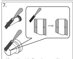
$\cdot$  After cutting, take file and remove all burrs. Try and bevel edge.
