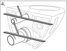
· With a ruler, against the back of the bowl, on top of pipe, mark as shown.
