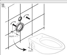
· Use slotted end of thread bolt to adjust in or out. Do not damage the thread.
