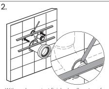
· With a ruler, against finished wall, on top of pipe, mark as shown.
