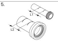
· Measure distance between both lines on pipes. Take measured distance, deduct from bald end of pipe and cut pipes as shown in step 6. This will allow some tolerance to recut if necessary.
