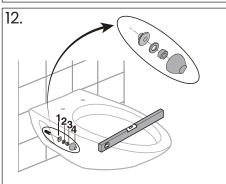
· Install with mounting hardware and ensure toilet bowl is level.
