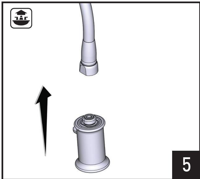
Install wand to upper connection of pulldown hose (**H**).
