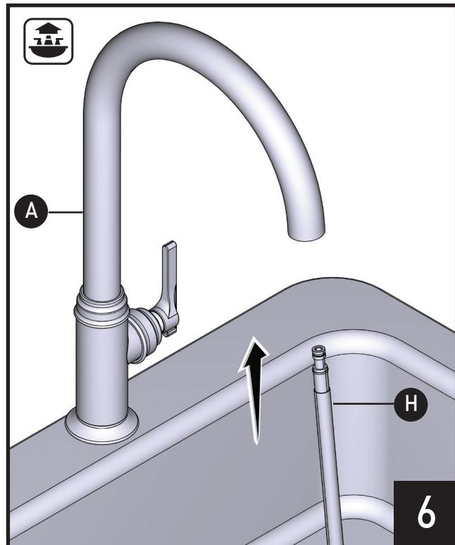
Insert small end of Pulldown Hose (**H**) into spout and feed through Faucet (**A**).
