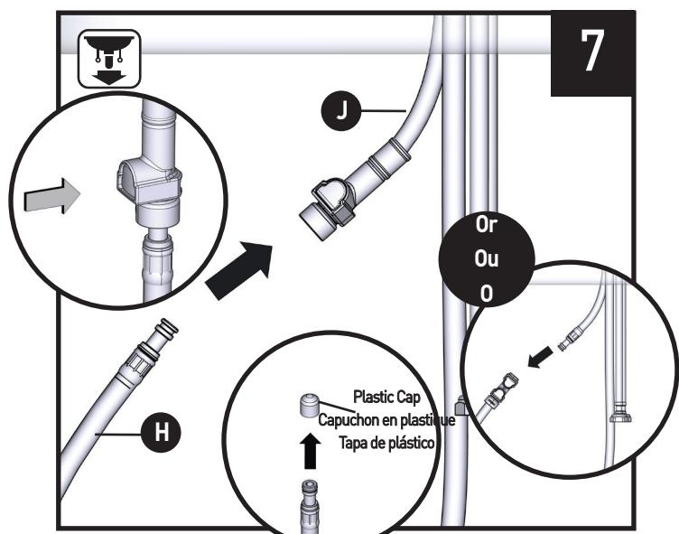
Remove and discard the plastic cap from the end of the Pullout Hose (**H**).
