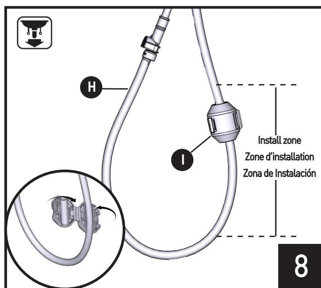
Install Hose Weight (**M**) between the bottom of the hose curvature and white tape of Pullout Hose (**I**). See above for recommended install zone locations.
