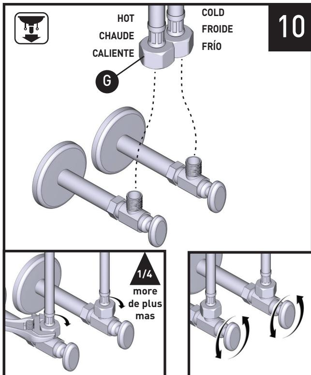
Attach faucet supply lines (**G**) to shut off valves. Tighten by hand, then 1/4 turn more with adjustable wrench. Turn on water and check for leaks.
