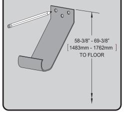
Drill necessary holes into mounting surface and secure Mounting Bracket to surface using appropriate hardware, being sure to torque to manufacturer's specifications.
