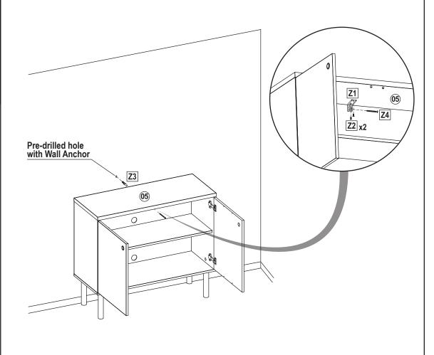
**IMPORTANT:** This unit is meant for drywall/stud mounting. If walls are concrete, brick or plaster, consult a professional.
