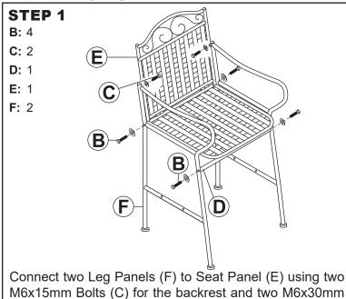
Bolt Sets (B) for the seat. Affix Support Bar (D) to the front of the leg panels, just below the seat, using two M6x30mm Bolt Sets (B).
