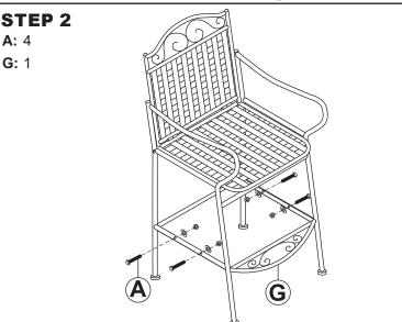
Secure Footrest (G) to the bottom of the leg panels using four M6x40mm Bolt Sets (A).
