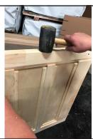
7. Once you've finished gluing the parts, carefully add the remaining side rail (part 8). Start by lining up the top rail and position the side rail so that all the parts fit into the corresponding slots. Using a rubber mallet, gently tap the rail down so the parts and rail fit snugly together.
