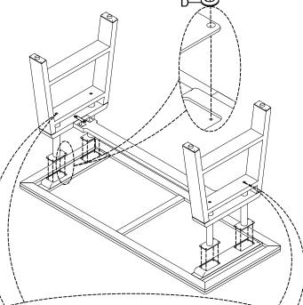
Loosen this bolt to adjust the mending plate of the metal tube to align with the groove/cutout on the tabletop, then tighten all the bolts.
