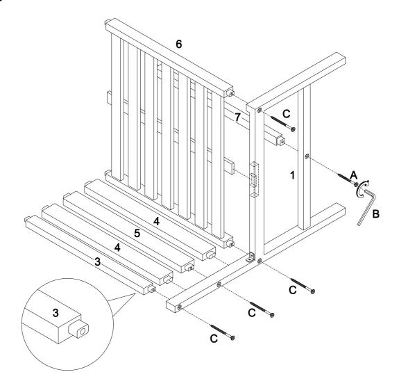
Insert part (4) into part part (1) as per diagram. Using bolt (A) insert into part (1) to part (7) ,and using bolt (C) into part (1) to parts (3,5,6) with hex key (B) as per diagram. Note: do not fully tighten all the bolts .
