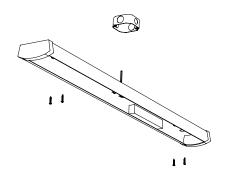
If mounting to junction box, place fixture against junction box and install two (2) screws through junction box mounting holes and into junction box mounting tabs.
