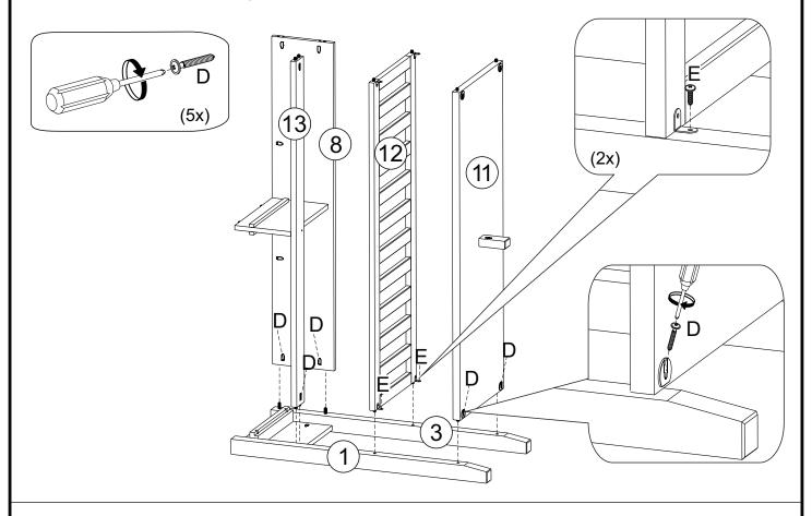
$Step \ 6^{\,\,\text{Use Screw D (x5) to attach parts 11 and 8 to legs 6 and 4. Use Screw E (x2) to attach Bracket G to parts 4 and 6.}$
