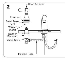
Sidevalve to be installed from underside of work surface as shown.
