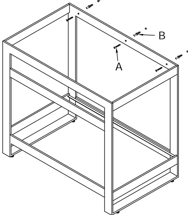
1. Place the stand upright in the desired location and level using the height adjusters built into the bottom of the stand.
