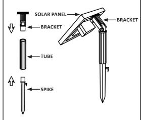
**6.** Insert the spike into the ground. Position the solar panel to face south (in the northern hemisphere) to make the most of daylight hours. It is important to angle the solar panel towards the sun when the sun is at its highest point. Ensure trees, shrubs, or buildings do not shade the solar panel.
