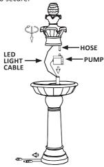
**4.** Fill the fountain with water, ensuring the pump is completely submerged during operation; approximately 1.5 gallons.
