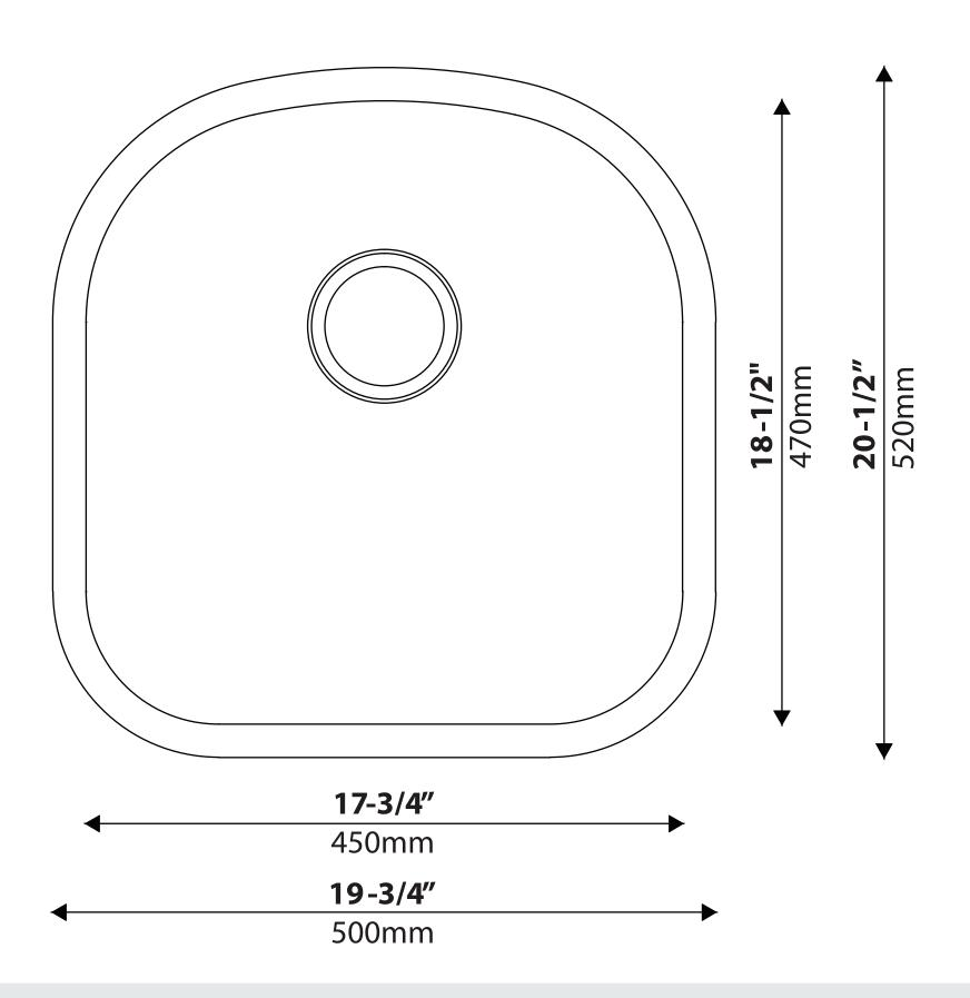
NOTE: Cutout template is provided as a guide ONLY and must be checked against actual sink to verify correct fit.
