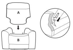
**Step3** Attach the lead wires found at the bottom of motion back to the lead wires at the rear of seat. The headrest leadwires are yellow to yellow. Make sure to close the clip locks to assure the connections will not come loose during use.
