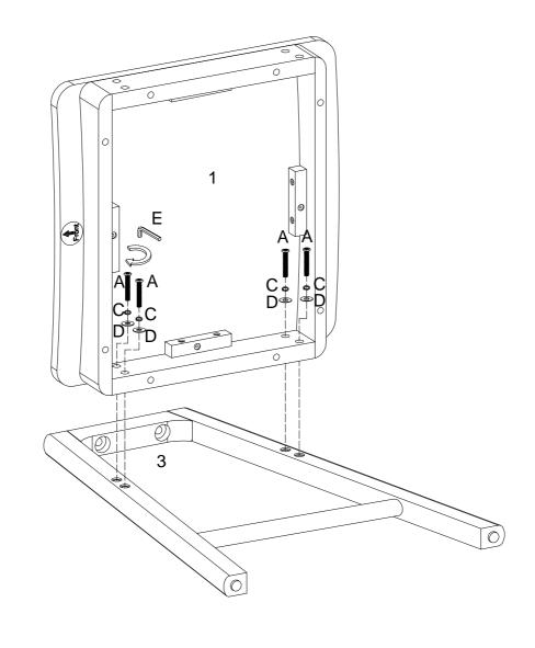
Now, repeat the process for the other side. Secure the Stool Seat (1) to the Right Leg Frame (4) using the Bolt (A), Lock washer (C), and Washer (D). Tighten with the Hex key (E).
