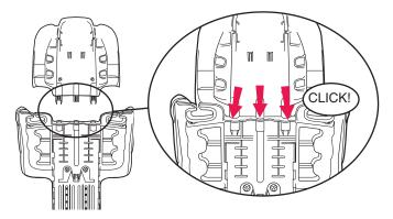
2. Install adjustment handle. Align tabs on adjustment handle with the slots on the back of the headrest. Press adjustment handle against the back of the headrest and slide upward until the tabs click into place.
