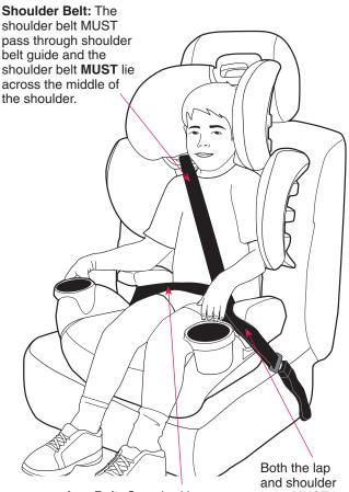
Lap Belt: Stretched low and snug across the child's hips, and fastened into the buckle. Both the lap and shoulder belts **MUST** be positioned under the armrest on the Booster Seat.
