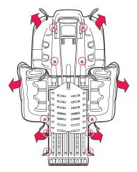
2. Remove the seat pad from the base. Disconnect elastic loops from the hooks on the back of the base. Disconnect retainer clips from the front of the base. Remove the seat pad.
