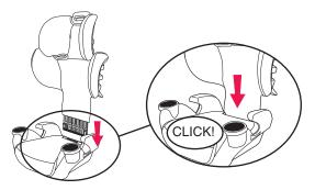
7. Check your work. Inspect the Booster Seat. Pull up on the headrest to make sure is securely attached to the backrest. Make sure the seat pad is hooked into place. Pull on the backrest to make sure it is securely attached to the base. Repeat any assembly steps as necessary.
