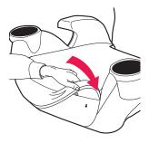
6. Install the backrest assembly. Position the base under the backrest assembly. Slide the backrest assembly onto the base. Make certain the backrest assembly locks into place with an audible click.
