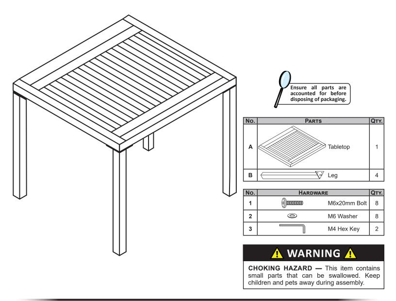
Tip: Always fully insert the hex key inside designated notch of the bolt.
