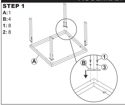
Lay Table Frame (A) face-down on a soft, clean surface.
