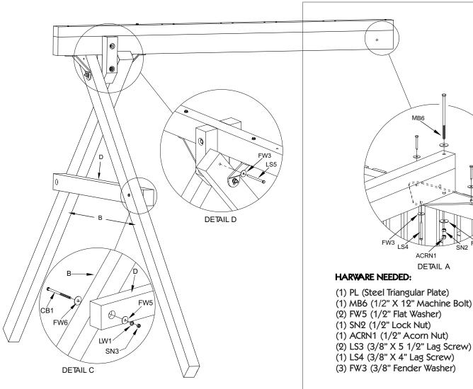
Before raising the headbeam, determine from Detail A or B how the headbeam attaches to the playset and the hardware needed based on the type set you purchased. Place the hardware needed to attach the headbeam up in the playset so it will be handy. Attach Steel Triangular Plate (PL) to the safety rail using LS3 and FW3.
