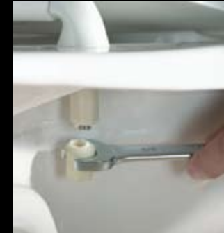
Using a 5/8" wrench, alternately tighten until lower portions shear off.
