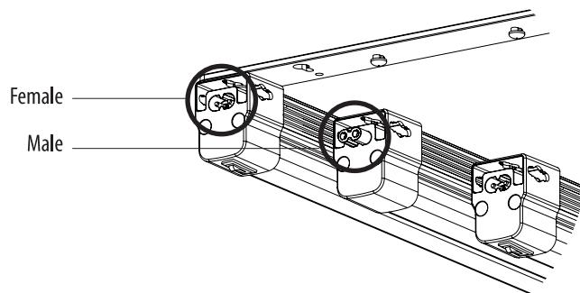
**3** Use the above assembly as a template. Place against the ceiling and mark mounting holes.
