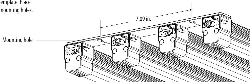
**4** At the marked locations, drill holes for the screw or anchor as appropriate.
