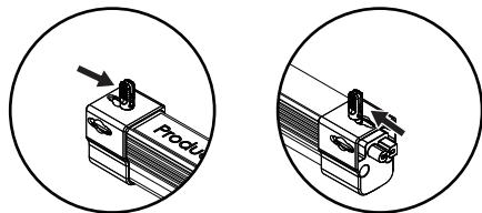
**4** Slide the 6 in. hanging cables into the cable clips.
