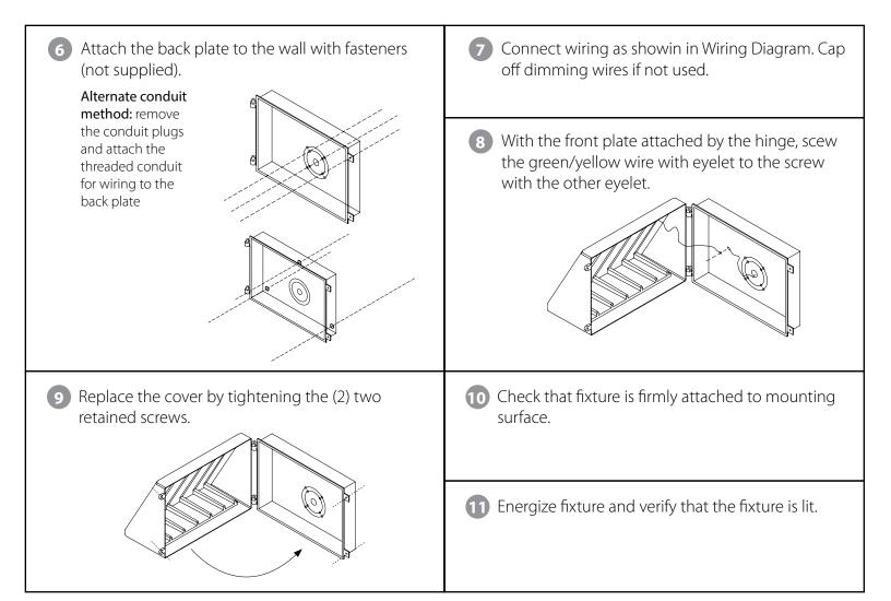
**IMPORTANT:** To weather-proof your outdoor installation, be sure to seal all mounting points, wire inlets, and penetrations (Conduit, Plugs, etc.) with silicone sealant.
