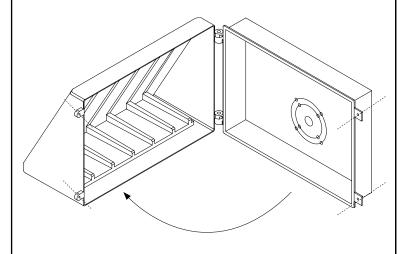
5 Open fixture and drill out the holes for mounting to a 4/O J-Box or 3-wall with diameter of 0.28".
