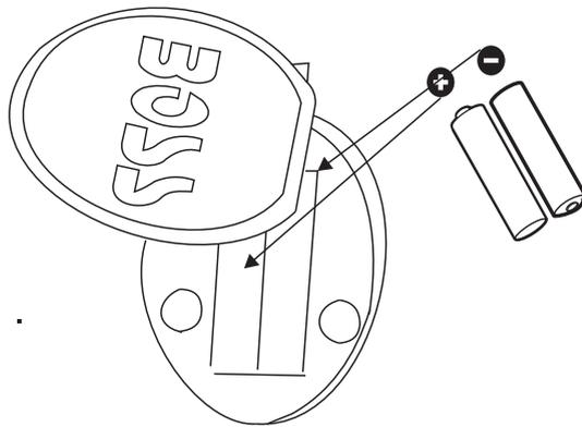
Insert two AAA type batteries (not included). Be sure to note proper polarity when installing the batteries.
