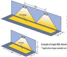
Example of multiple **INDL** luminaires illuminating a 3' path of egress.
