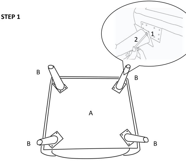
Place the Chair (A) upside down on a flat smooth surface. Attach Legs (B) to the bottom of the Chair (A) with Bolt (1). Use Allen Key (2) to tighten.
