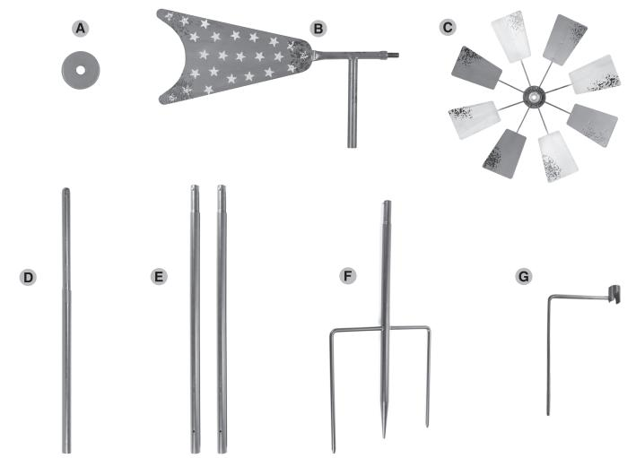
1. Attach wheel (C) face-out on fin (B) by inserting threaded portion through center hole of wheel. Next, screw on cap nut (A) by turning it to the right until it is firmly tightened.
