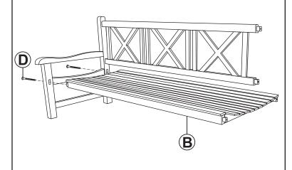
Secure Backrest (C) to the right Side Panel (A) using two 6cm Bolts (D).
