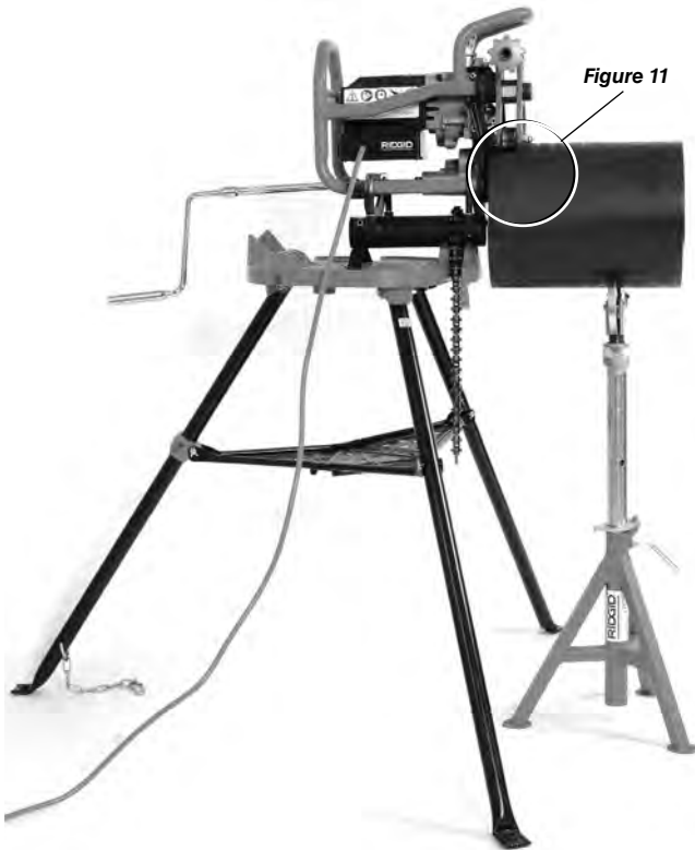
Figure 12 – Machine fixe, tuyau court, un porte-tubes
