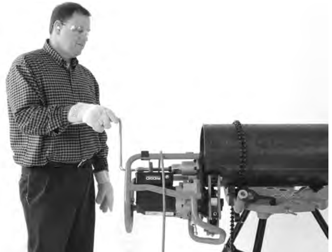
Figure 20B – Bevelling Operation (Fixed Workpiece/Moving Beveller)
