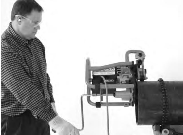
Figure 20A – Bevelling Operation (Fixed Workpiece/Moving Beveller)
