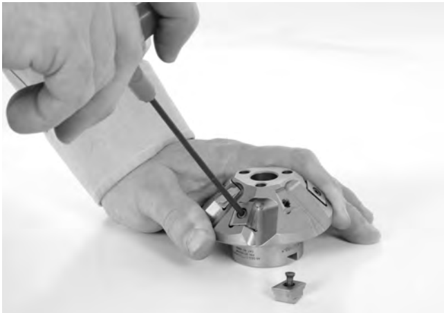
Figure 24 – Replacing Cutter Inserts
