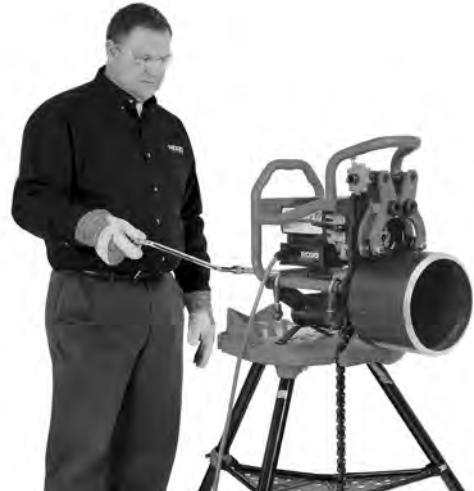
Figure 20C – Bevelling Operation (Fixed Beveller/Rotating Pipe)
