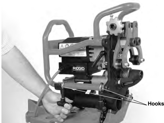
Figure 9 – Securing Beveller to Adapter
