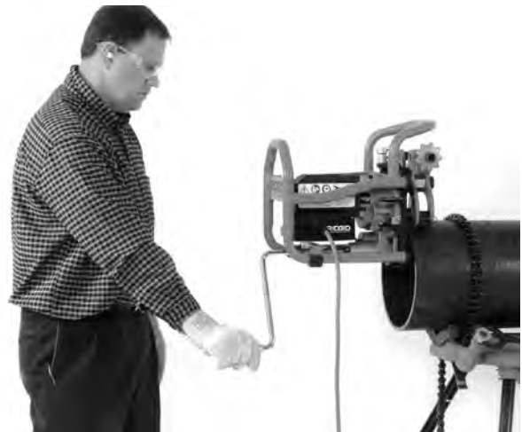
Figure 19 – Proper Operating Position
