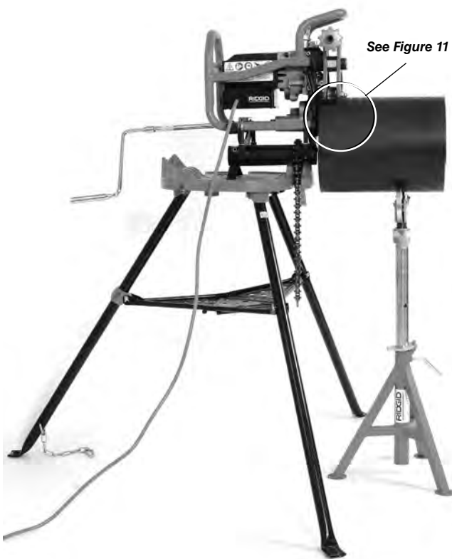
Figure 12 – Fixed Beveller, Short Pipe, One Pipe Stand
