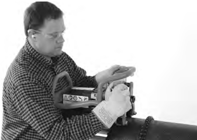
Figure 17A – Hand Tighten Clamp Screw
