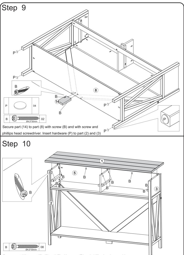
Secure part (1) to part (2), (3) and (5) with screw (B) and phillips head screwdriver.
