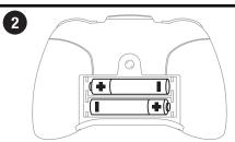
**2.** Install new batteries as shown in the polarity diagram (+/-) inside the battery compartment.
