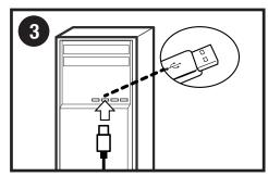
**3.** Plug the charging cable into a 5V DC computer outlet.
