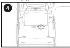
**4.** Charging LED indicates charging. Solid ON for charging and turn OFF when fully charged.
