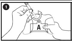
1. Open the battery door with a screwdriver (A). If used batteries are present, remove these batteries from the unit by pulling up on one end of each battery. DO NOT remove or install batteries using sharp or metal tools.
