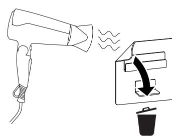
If you need to remove the installed adhesive, you can use a hair dryer to heat the adhesive surface and slowly separate from mounting surface.
