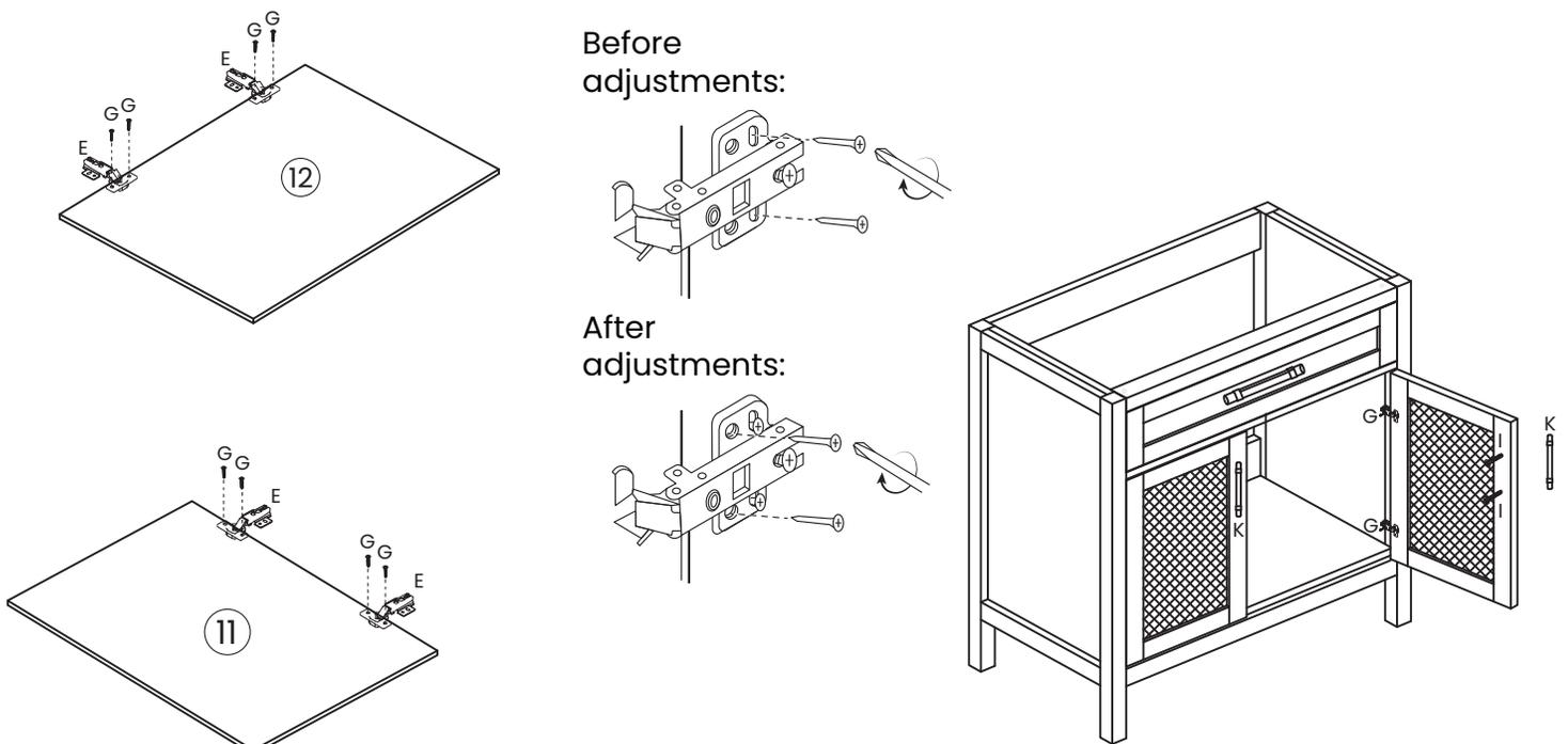
**Hinge/Door Adjustment & Realignment**
