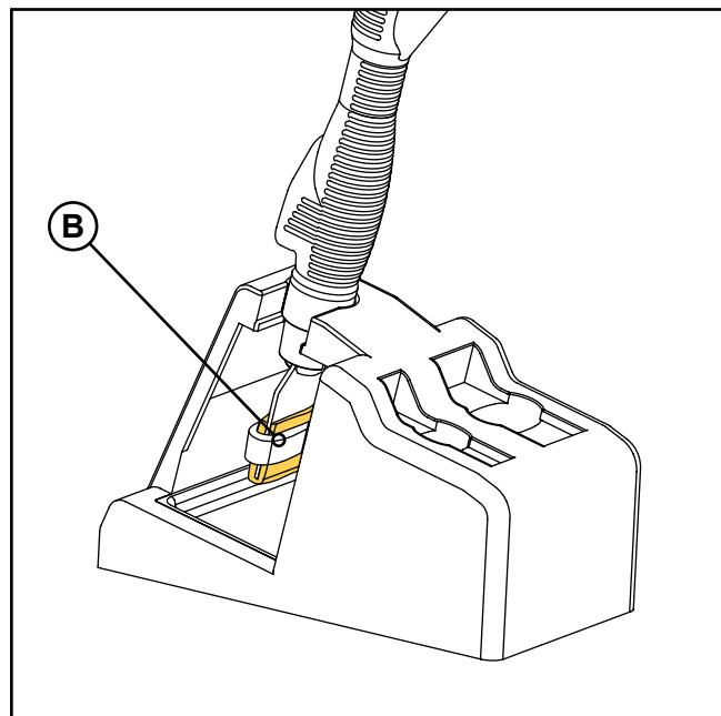
The holder is designed to stow the mini wand with a brush (A) or an insert (B) installed.
