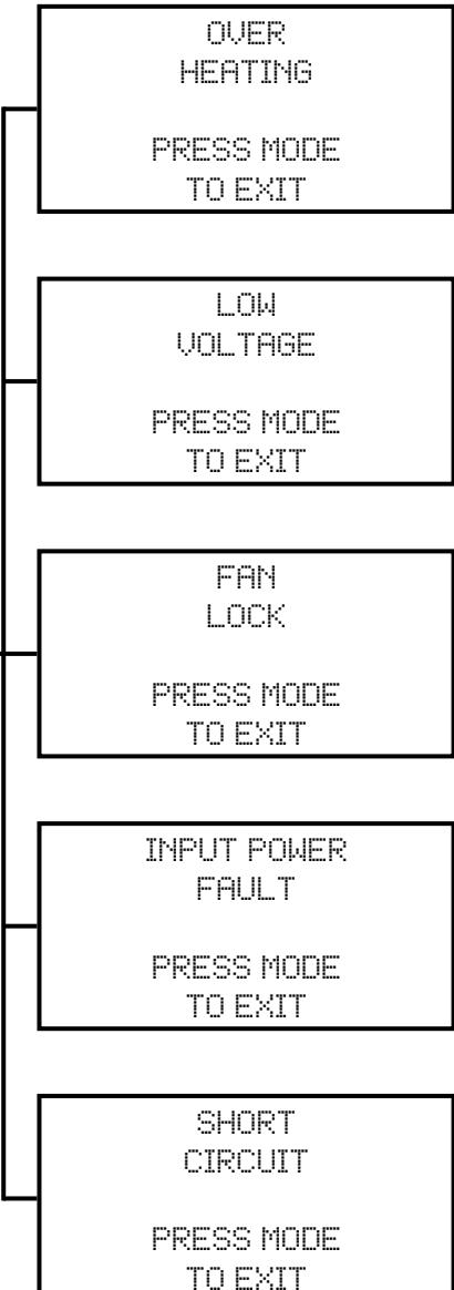
The thermal protection system has been activated (see chapter 1.2). It will not be possible to restart the device until it has cooled down.
