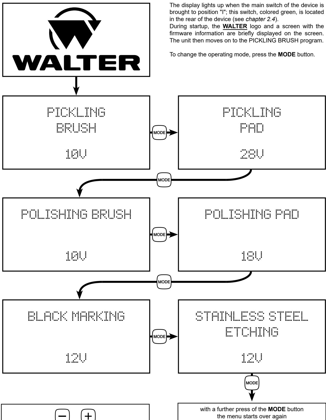
Regardless of the program selected, the – and + keys can be used to increase or decrease the working voltage (in 1-volt increments).
